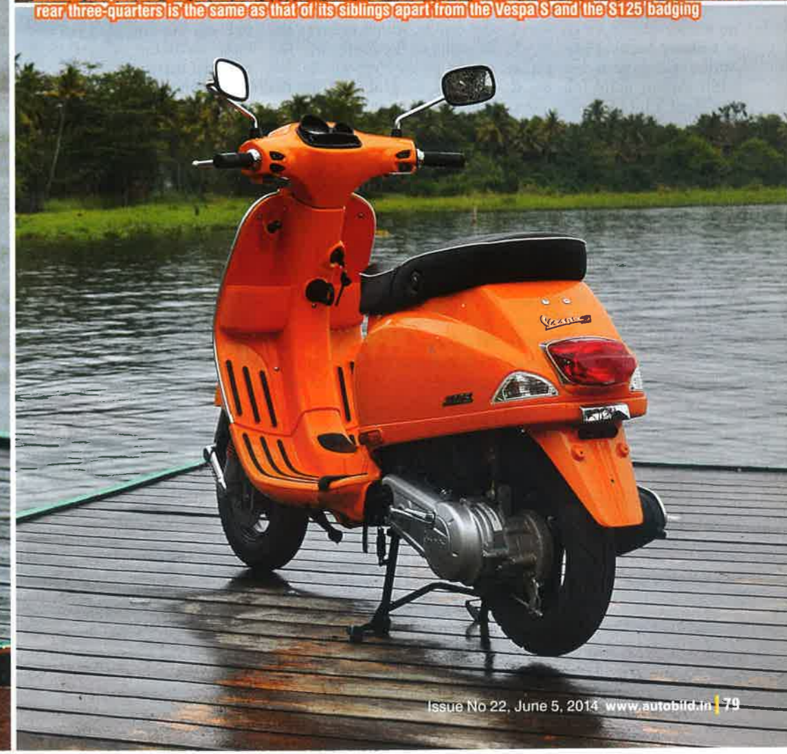
Above: Vespas are one of the few scooters that still make use of a monocoque chassis design. Below: The rear, three-quarters is the same as that of its siblings apart from the Vespa S and the S125 badging
