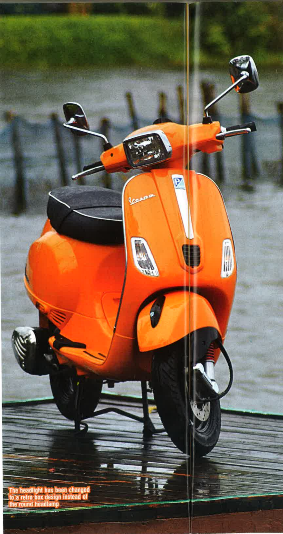
Above: Vespas are one of the few scooters that still make use of a monocoque chassis design. Below: The rear, three-quarters is the same as that of its siblings apart from the Vespa S and the S125 badging
